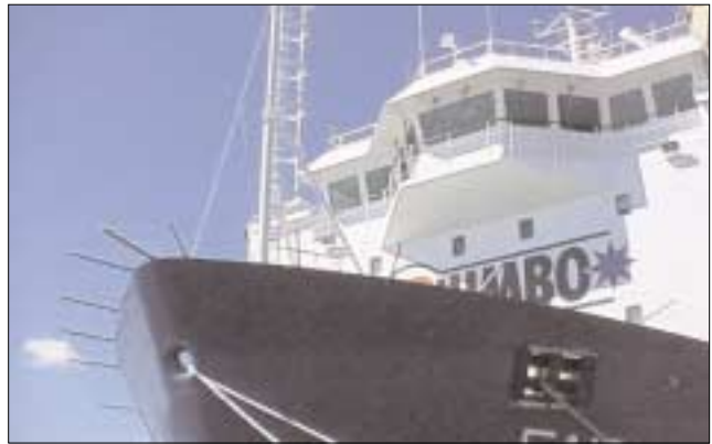
An electric fence on a ship - will all ships need these in future to be adequately defended against pirates? Photo courtesy Secure Marine
