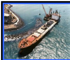
Sergio Zakariadze: grounded whilst entering San Juan, Puerto Rico, in November 1999. Salvors lightered 10,000 tonnes of cargo and then refloated the casualty.
