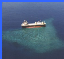
Pollution threat: salvors reduced leakage from a fuel tank and then refloated the 6,700 dwt Partner, following her grounding on a reef in Papua New Guinea.
