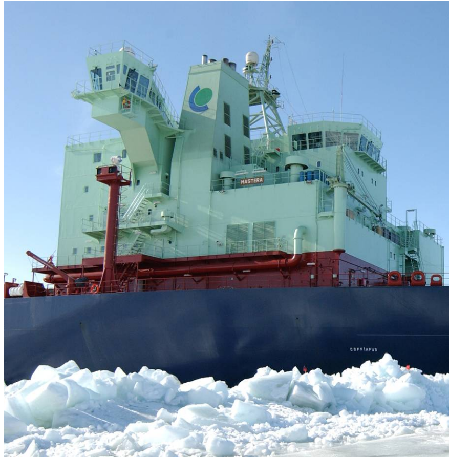
Figure 7: Close up view of deck and wheelhouse of Neste Oil double-acting tanker showing enclosed bridge wing arrangement (photo courtesy of Neste Oil)
