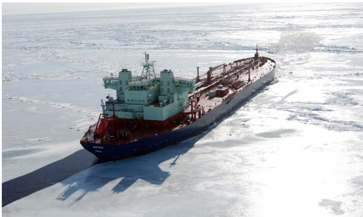
Figure 4: Mastera : double-acting tanker operating in astern mode in first year Baltic ice (courtesy of Neste Oil)
