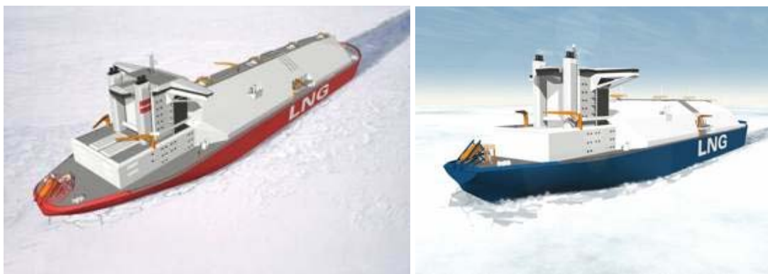
Figure 6: Artist's impressions of large double-acting LNG ship design concept developed for ArcOp project
