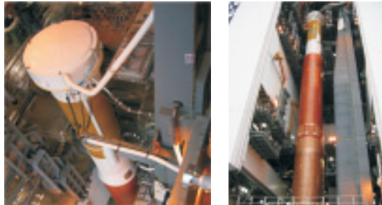
Atlas V Before Solid Rocket Boosters Installation (Height With Fairing Installed Is 59.2 Metres)
