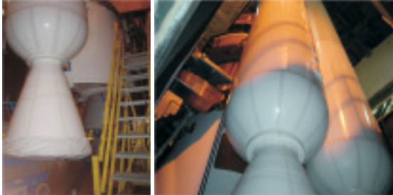
Two (of Three) Solid Rocket Boosters After Installation Onto The Main Core Booster
